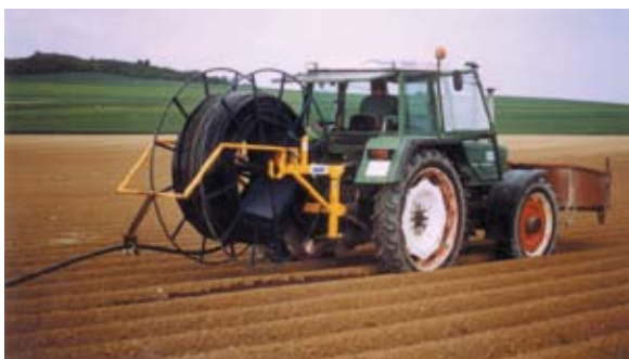
IrriStand laying operation
