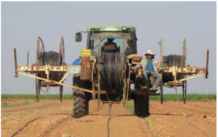
Three reels laying machine, 13000-20,000m
